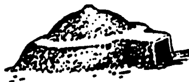
Earthlodge made of a wood frame with earth-covered walls
