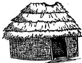
Wattle and Daub made of a wood frame, vines and clay
